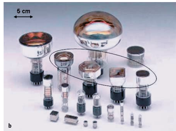
Fig. 1.9. a The basic design and operating principle of PMTs and scintillation detectors. b Photographs of PMTs. The PMTs circled are typical of those used in gamma cameras
