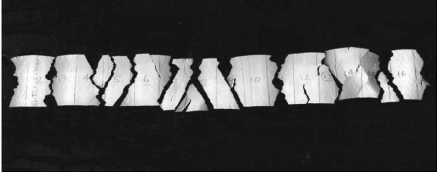
Fig. 8.17. Fragments from one magnetic expanding cylinder test on 6061-T6 aluminum [Weisenberg and Sagartz, 1977]
