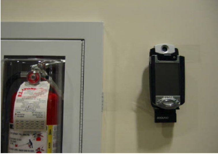
Fig. 6. IPAQ handheld computers equipped with a camera and a wireless adaptor serve as our sensor nodes. They are mounted on the walls in our office building.
