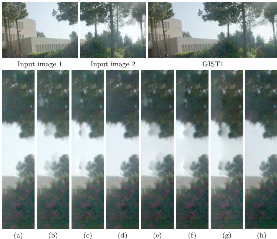
Fig. 5. A comparison between various image stitching methods. On top are the input image and the result of GIST1 under \ell_1 . The images on bottom are cropped from the results of various methods. (a)-Optimal seam, (b)-Feathering, (c)-Pyramid blending, (d)-Optimal seam on the gradients, (e)-Feathering on the gradients, (f)-Pyramid blending on the gradients, (g)-Poisson editing [10] and (h) GIST1 - \ell_1 . When there are large misalignments, optimal seam and GIST1 produce less artifacts.
