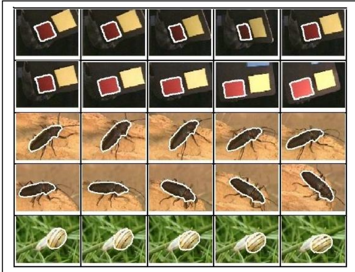
Fig. 4. Four experiments: (1) tracking of circles that change the colour; (2) tracking an object surface with different orientations and illumination; (3) tracking an insect in real environment; (4) tracking a snail in real environment
