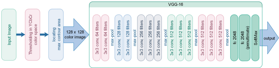
Fig. 1. Processing pipeline of our TFS sign recognition.
