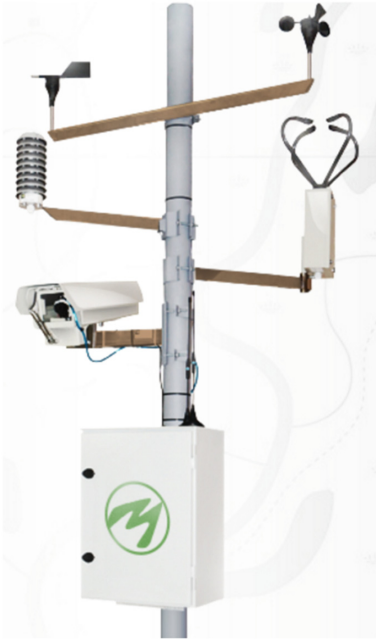
Fig. 1. RWIS and its sensors
