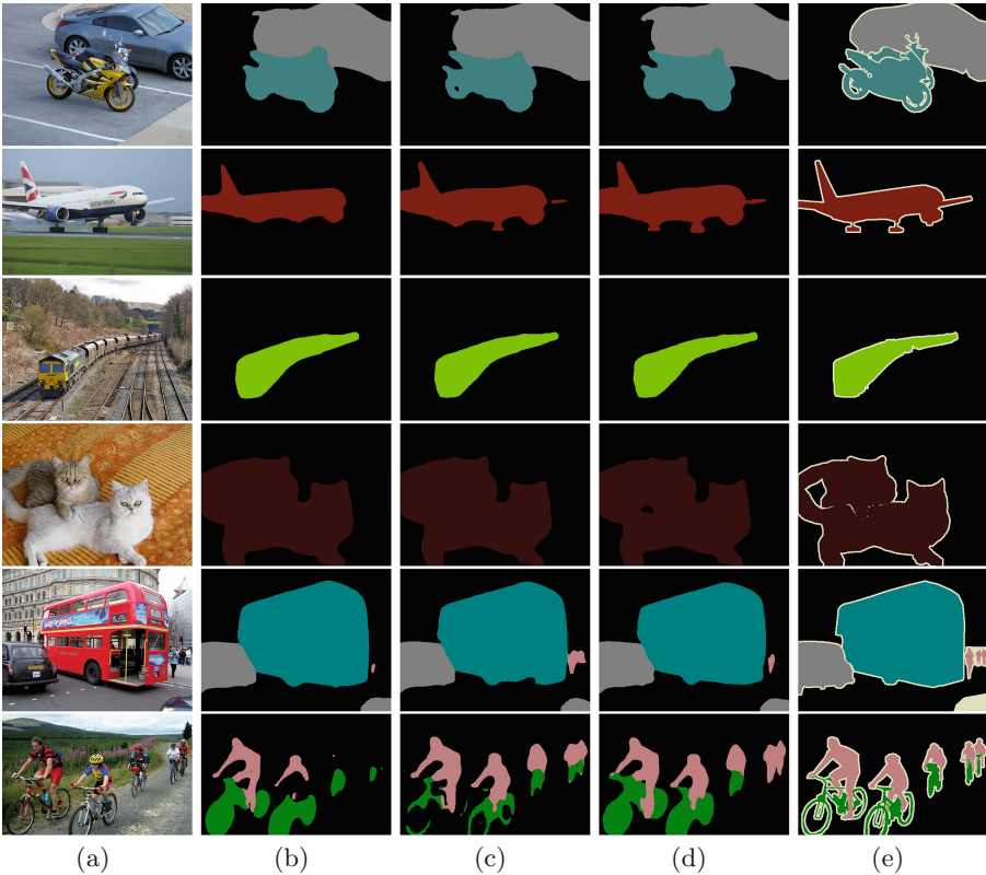
Fig. 4. Qualitative comparison of the results obtained with the three different supervision strategies. (a) Original image. Segmentation obtained by weak bounding box annotations (b), based on the semi-supervised setting (c), and by pixel-level annotations (d). (e) Ground-Truth segmentation.
