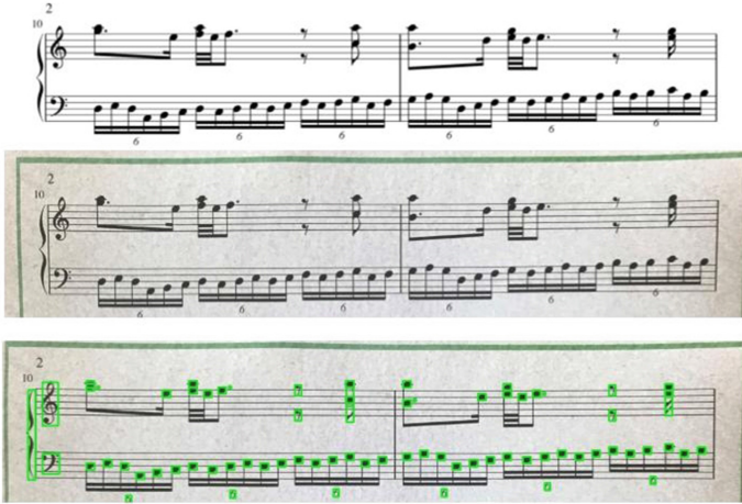
Fig. 10. Top: part of a synthesized image from DeepScores ; middle: the same part, printed on old paper and photographed using a cell phone; bottom: the same image, automatically retrofitted (based on the dark green lines) to the original image coordinates for ground truth matching (ground truth overlaid in neon green boxes). (Color figure online)
