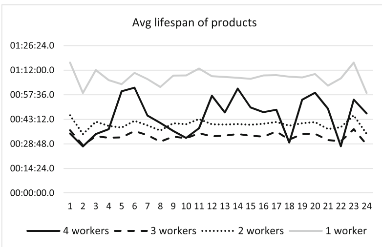
Fig. 9. The average lifespan of products for model S2, with a different number of maintenance workers
