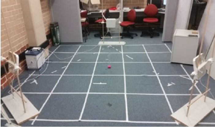
Fig. 7.2 Platform setup and Monza 4D “target tag in the middle of the platform”
