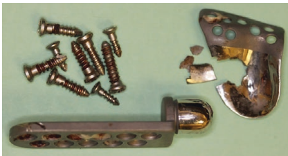
Fig. 8.9 Potential complications of these devices are metallosis and fracture of the fossa component
