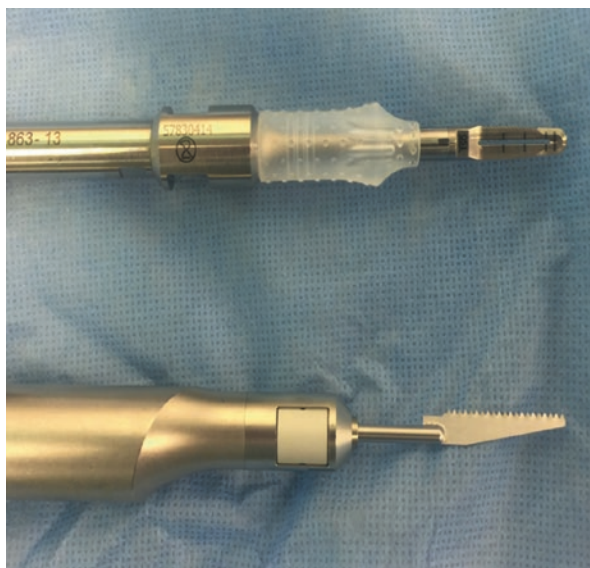
Fig. 9.11 The BoneScalpel (top) versus a reciprocating saw (bottom). The BoneScalpel is a piezoelectric device that preferentially cuts the bone instead of soft tissue. The device has been shown to significantly reduce intraoperative bleeding during TMJ replacement surgery
