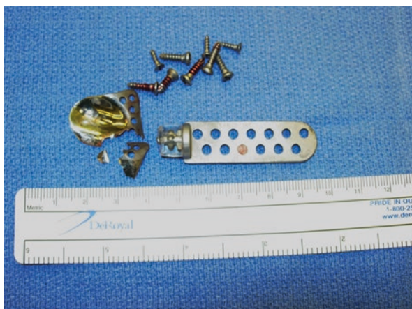
Fig. 9.3 Fracture of the fossa component in a Christensen stock TMJ total joint prosthesis. The patient underwent explantation of the entire prosthesis and eventual reconstruction with a custom prosthesis
