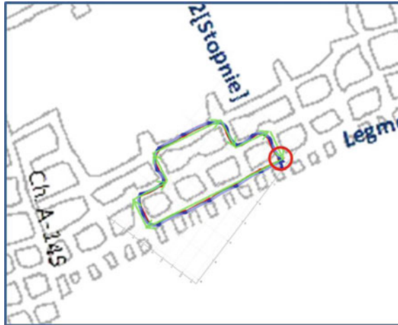
Fig. 5 Route correlation experiment. Green arrows denote segments of planned route, blue data is a set of versors for the measured points, and red circle is the point of start and finish
