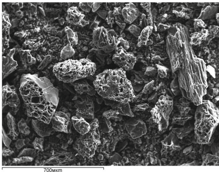
Fig. 1 SEM micrograph of the special coke fines sample
