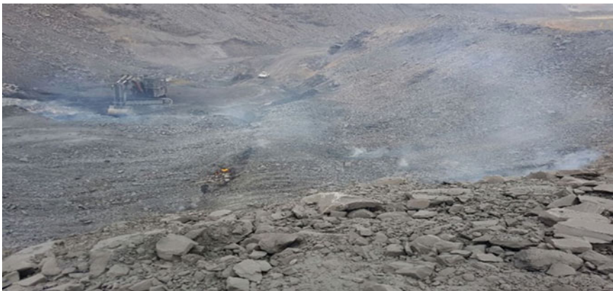
Fig. 2 Symptoms of self-heating at mine face at Khwezela Mine (Bokgoni Pit), Witbank, South Africa (Onifade and Genc 2018b, c, d; Onifade et al. 2018)
