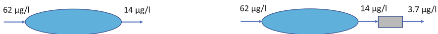
Fig. 1. To the left a wet pond treating the stormwater and to the right a wet pond combined with a smaller underground retention filter basin.
