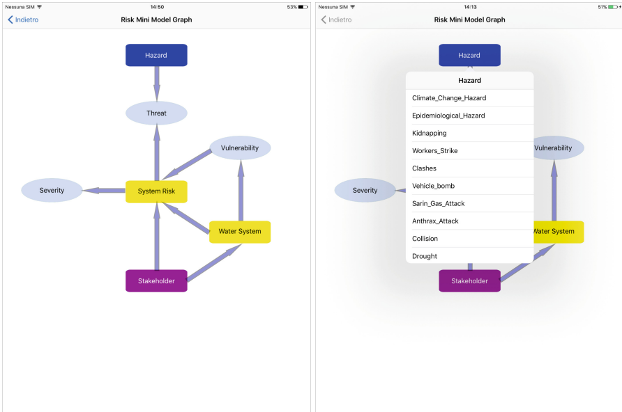
Fig. 4. Example usage of the ICE app. The left part shows a screenshot of the risk mini model pattern still to be instantiated. The right part shows a screenshot where hazard is selected by clicking on the corresponding diagram element.
