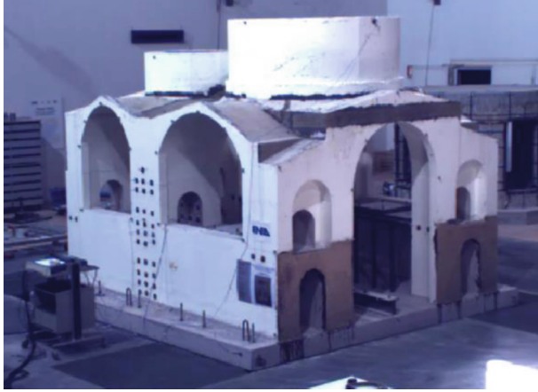
Fig. 2. The mockup of Hagia Irene, tested on shaking table at ENEA Casaccia Research Center (from the original ppt Video 1_11 [9]).
