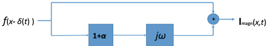
Fig. 1. Temporal filtering applied to each pixel time history. Cut-off frequencies have to be chosen carefully in order to enclose the band of the phenomenon to be analyzed and exclude other frequencies.
