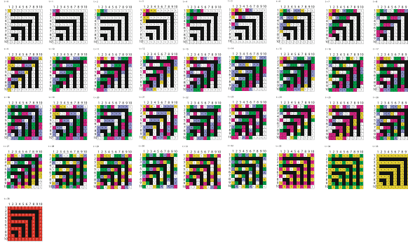
Fig. 10. Snapshots of the synchronization processes on a 2D array of size 10 \times 10 , including 4 defective zones
