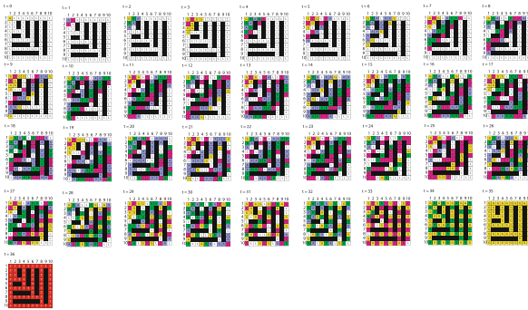
Fig. 11. Snapshots of the synchronization processes on a 2D array of size 10 \times 10 , including 7 defective rectangle zones
