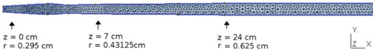
Fig. 2 A longitudinal cross-section of the 3D geometric shape of the tubing near the mouthpiece boundary used to construct the computational trumpet
