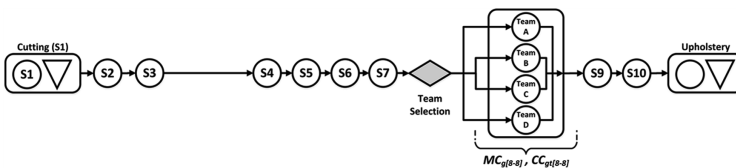
Fig. 2. Process flow with push control
