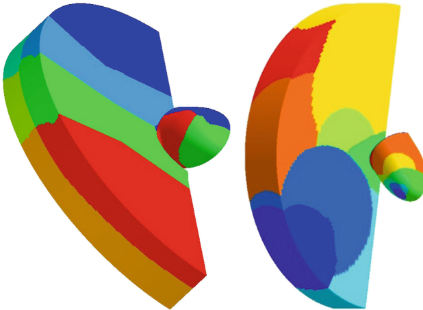
Fig. 2. Examples of decompositions: SCOTCH (left), hybrid (right)
