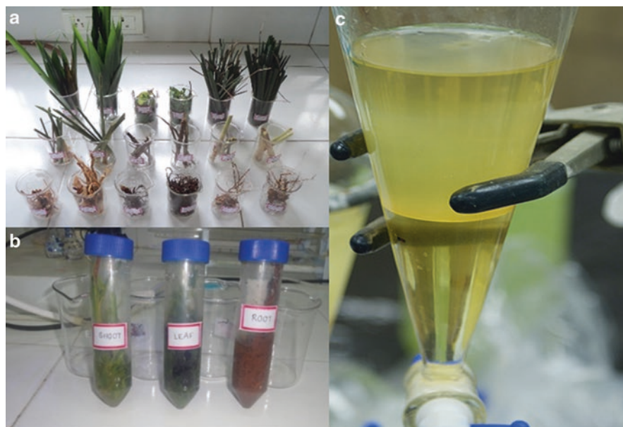
Plate 18.2 Extraction of endosulfan from plant parts. (a) Different parts of the plants selected, (b) treated plant parts in centrifuging tubes, (c) extraction in separating funnel
