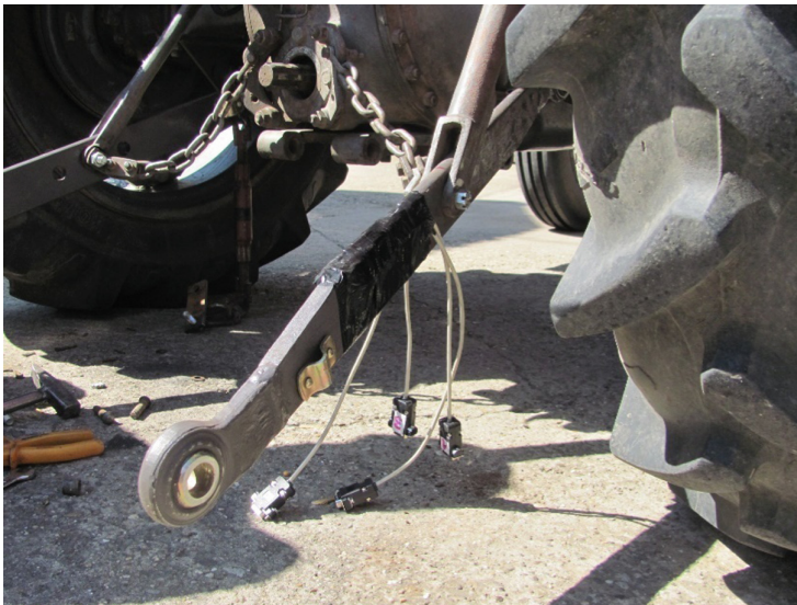
Fig. 5. Lower link with applied strain gauges on the tractor
