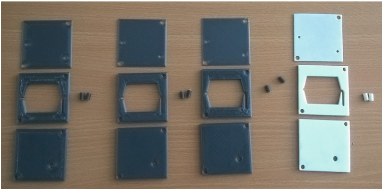
Fig. 9. All printed prototypes of PEM fuel cell reformer: (left to right) FDM 0.3 mm, FDM 0.2 mm, FDM 0.1 mm, SLA 0.1 mm.
