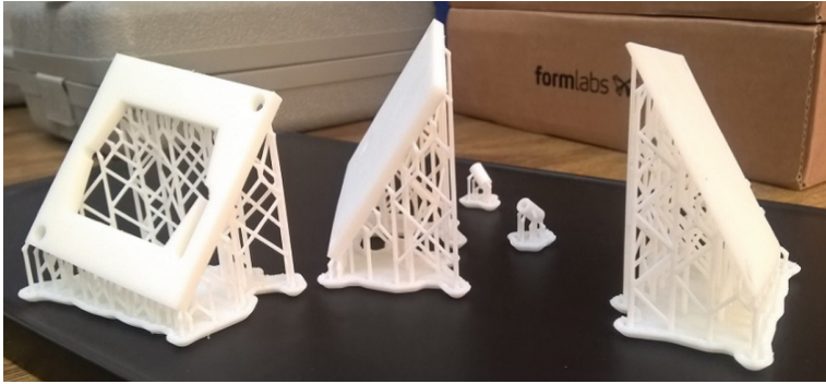
Fig. 8. SLA print of PEM fuel cell reformer.
