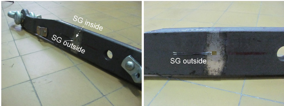
Fig. 4. Strain gauges position
