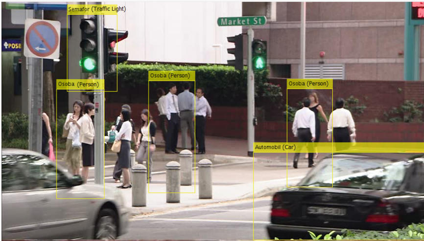
Fig. 12. Identified and recognized Pedestrians, Car and Traffic Light.
