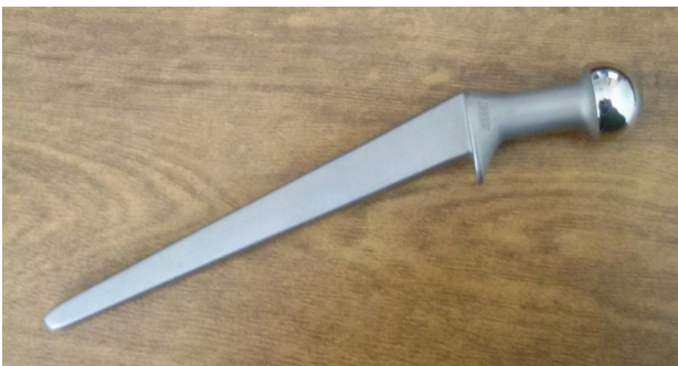
Fig. 3. Hip implant model made of CoCrMo alloy.
