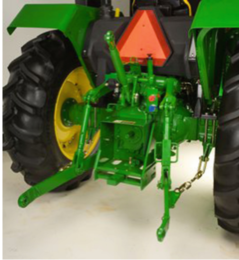
Fig. 1. Three-point hitch mechanism (TPH) [5].
