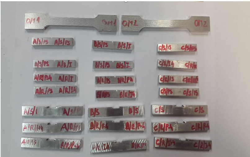
Fig. 4. Tensile specimens, impact test specimens and SENB specimens
