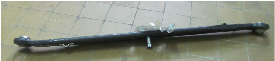
Fig. 2. Lower link of the TPH mechanism.
