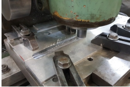
Fig. 1. Machine for FSW welding
