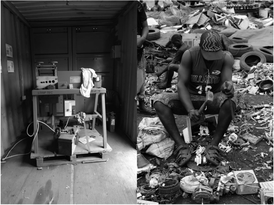
Fig. 3. Cable stripping machine (left) and electronics recycling (right) in the Agboghloshie scrap metal yard (Photos: SMART/Maja van der Velden)
