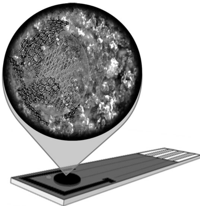
Fig. 20.3 A screen-printed glassy carbon electrode with working electrode modified with rGO-PEDOT:PSS composite for enhancement of electron transfer at the electrode-solution interface (Source: Reference with copyright permission)
