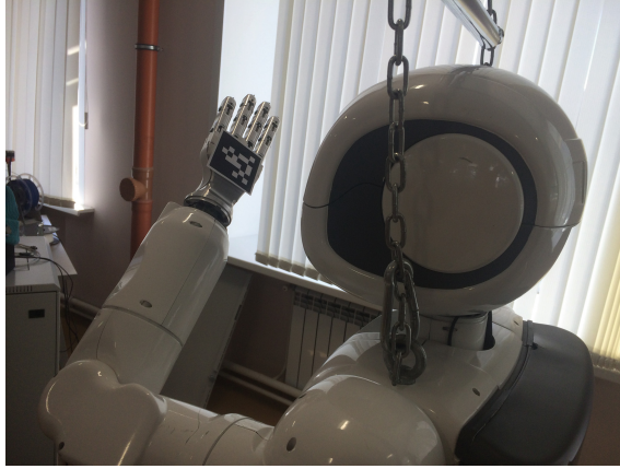
Fig. 6. Example of an experiment with AprilTag marker.
