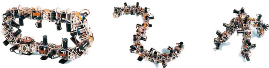
Fig. 1. Examples of different configurations of modular robot PolyBot (PARK, Xerox, USA): wheel, snake and walking configuration.
