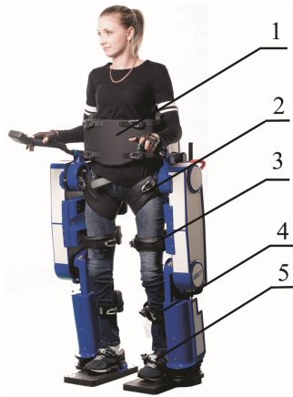
Fig. 1. General view of ExoLite exoskeleton with a user with fixed using connector pads; 1 – pads for torso connectors, 2 and 3 – pads for hip connectors, 4 – pad for shin connector, 5 – pad for foot connector.
