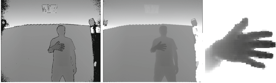
Fig. 3. Left: Input depth image, Middle: Depth image after depth hole filling, Right: Result of the hand tracking.
