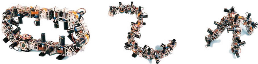
Fig. 1. Examples of different configurations of modular robot PolyBot (PARK, Xerox, USA): wheel, snake and walking configuration.
