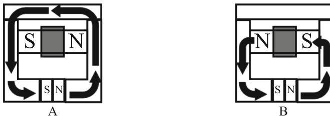
Fig. 4. The first prototype of the magnetic circuit: A – connection grip state; B – disconnection grip state.
