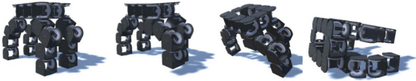
Fig. 9. Modeling of walking platform motion based on “cautious gait” scheme “1-2-3-4” where there is a loss of stability.
