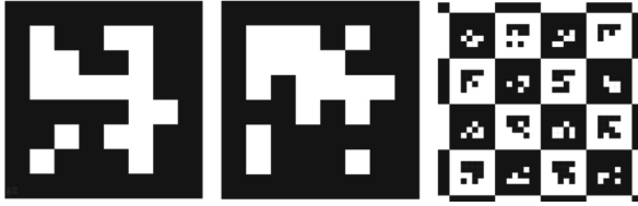
Fig. 2. From left to right: ARTag (ID 2), AprilTag (ID 4) and CALTag fiducials.
