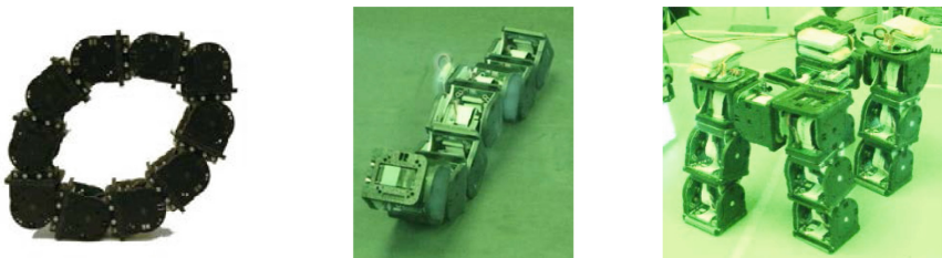
Fig. 2. Examples of different configurations of modular robot CkBot (Modlab, UPenn, USA): wheel, snake and walking configuration.
