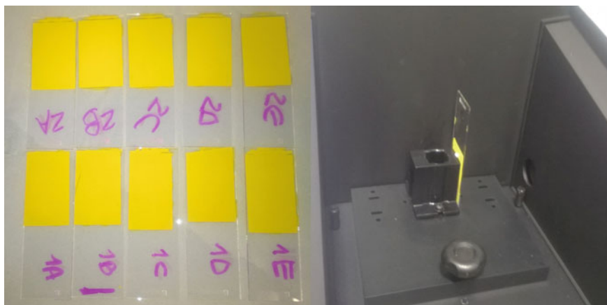
Fig. 3 Repeatability of coating method was assessed using UV-vis spectroscopy
