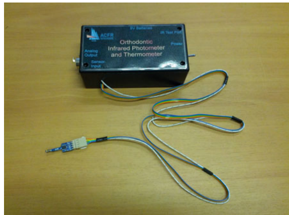
Fig. 6 The complete orthodontic infrared photometer and thermometer
