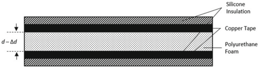
Fig. 6 Layered structure of the capacitive force sensor
