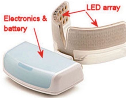
Fig. 4 Photograph of the OrthoPulse unit [11]
