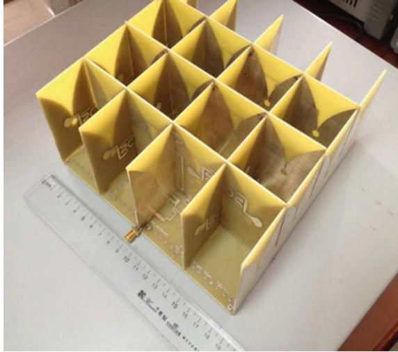
Fig. 4 Fabricated antennae system [23]
