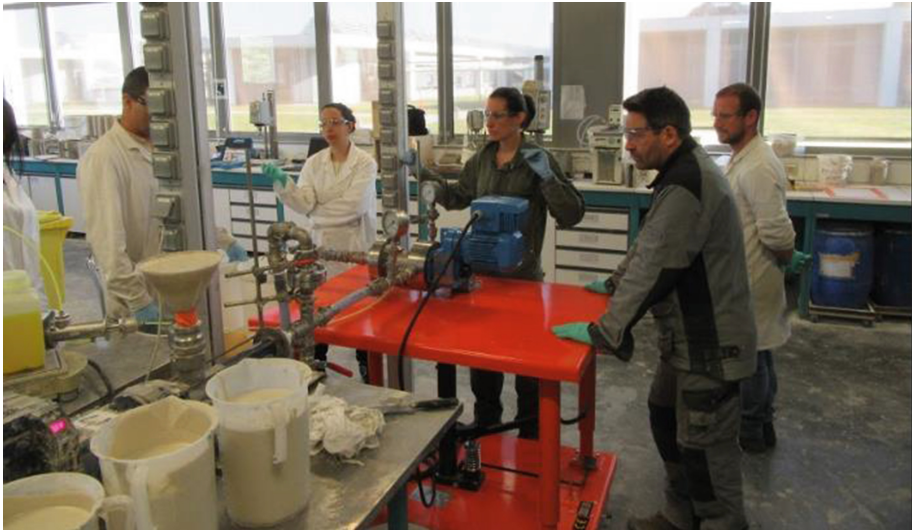
Fig. 2. Lab-scale extrusion system layout. Main pump can be seen on the left hand side, front. Secondary pump: left hand side, back. Mixer system in the middle. Material in buckets: C60
