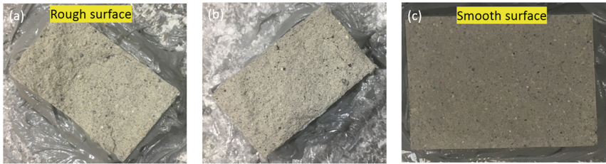
Fig. 5. Surface roughness of interface (a) MR = 2.0 (b) MR = 1.85 (c) MR = 1.60 geopolymer
