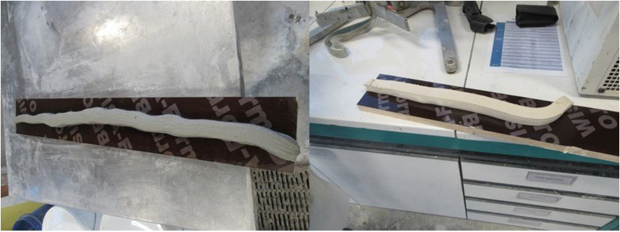
Fig. 8. Extruded samples of NAG3 formulation (left), and C60 formulation (right)
