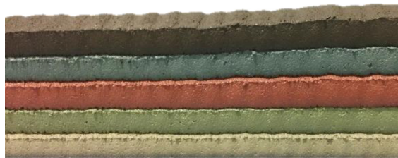
Fig. 6. Visualization of graded materials in construction-scale 3D printing using color concrete
