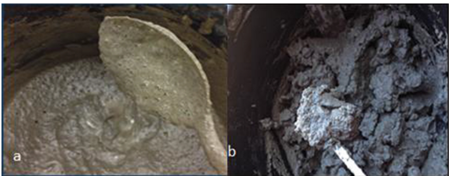
Fig. 1. Fresh state differences between classical (a) and extrudable (b) foamed concrete.
