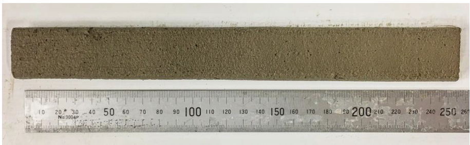
Fig. 2. The filament was extruded to evaluate the extrudability.
