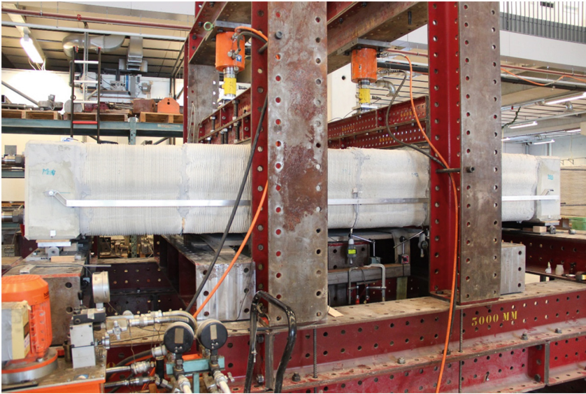
Fig. 14. Scale model in 4-point bending test set-up. Reproduced from [16].
