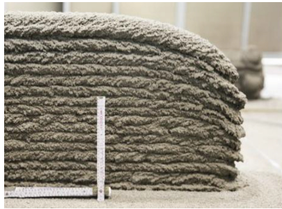
Fig. 3. Sacking on unsupported edges ( 180^\circ turns)
