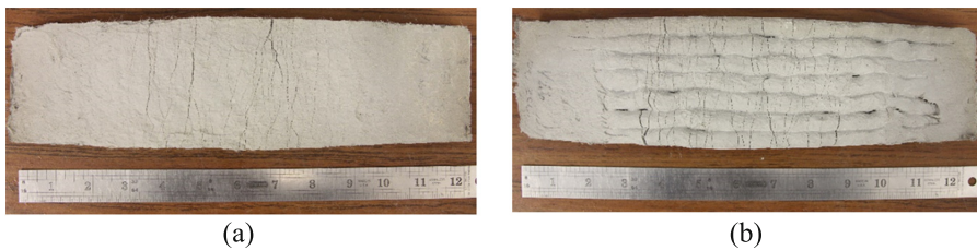
Fig. 10. Crack patterns in functionally-graded composite specimens tested under flexure: (a) S2 and (b) S3. Densely distributed microcracks are observed at the surface of the slab specimens.
