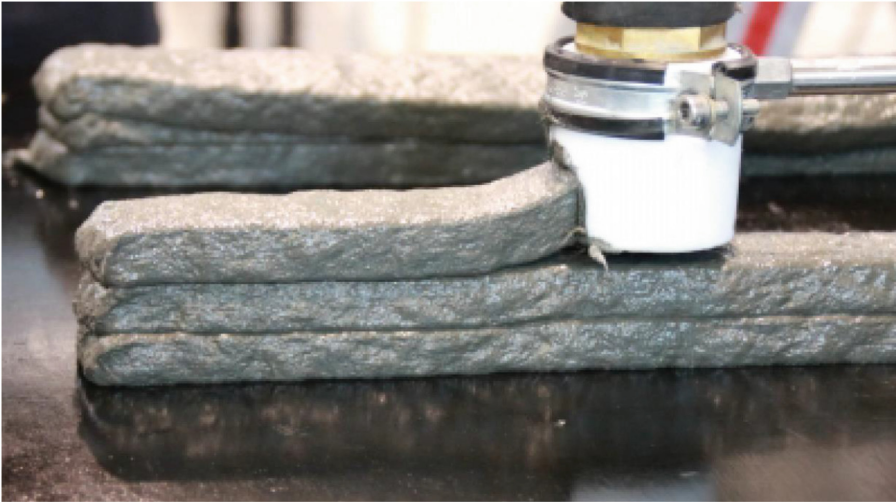
Fig. 4. Printing with SHCC Mixture B.
