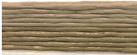
Fig. 4. Depositing 10 layers of printed filaments within 10 min indicates adequate buildability.
