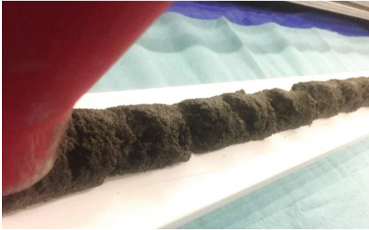
Fig. 2. Low print quality (tearing) of extruded layer caused by inappropriate workability
