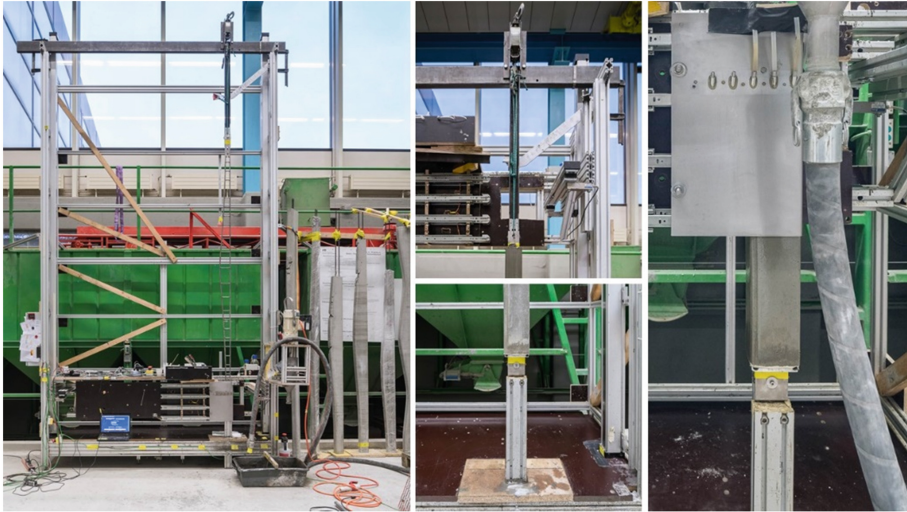
Fig. 7. (left) linear axis prepared for production, (bottom center) pretension attachment of rebar, (top center) rebar tensioned upwards, (right) beginning of slipping process
