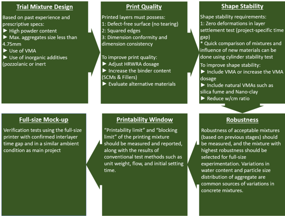
Fig. 1. Suggested procedure for performance-based testing of printing mixture at fresh state
