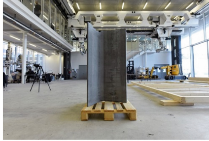
Fig. 9. The first thin folded concrete prototype produced with the SDC FS_2 Mix
