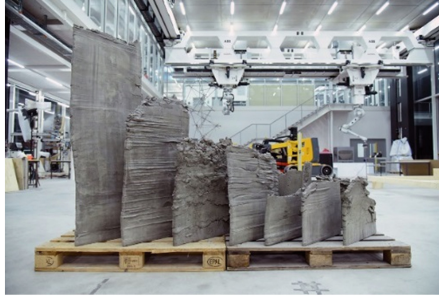
Fig. 4. The initial thin folded concrete prototypes using the SDC NEST Mix
