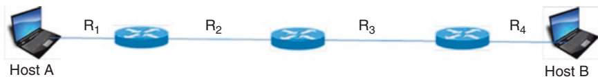
Fig. 2.9 Throughput for a file transfer from host A to host B with a single route
