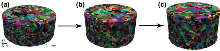
Fig. 7.10 Three 3D volumes of the measured microstructures a initial, b 6% strain, and c 12% strain. Colors correspond to an RGB mapping of Rodrigues vector components specifying the local crystal orientation [17]
