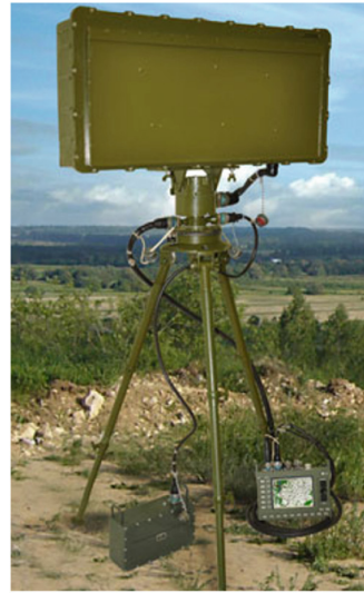
b) with an active antenna array and distributed gain
