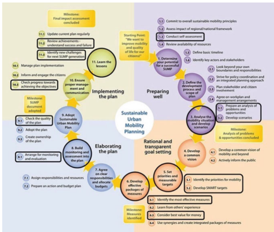
Fig. 10.1 Steps of the planning process for SUMP development. Source: Adapted by ELTIS (2017)
