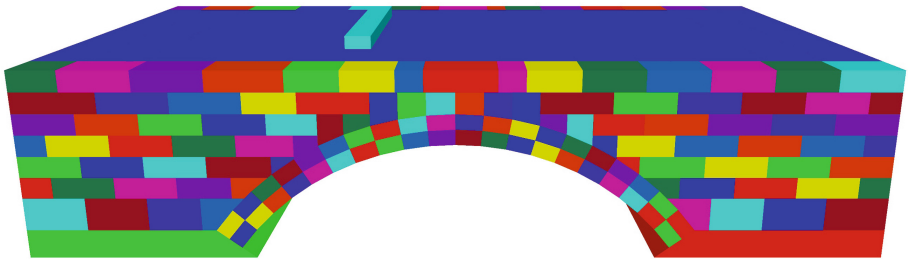
Fig. 1. 3DEC model – Bolton Institute Bridge
