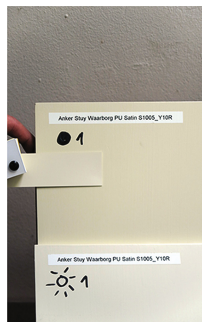
Fig. 11. Mock-up of the paint systems (yellowing) (© Ann Verdonck)
