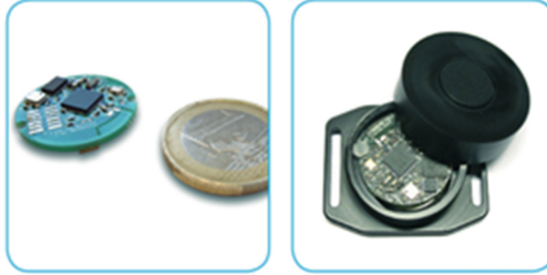
Fig. 2. VTT Tiny Node: a battery operated sensor board.
