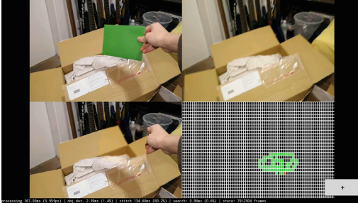
Fig. 9. Split view containing (from top left to bottom right): camera input, fill frame, (inpainted) output frame, frame store array
