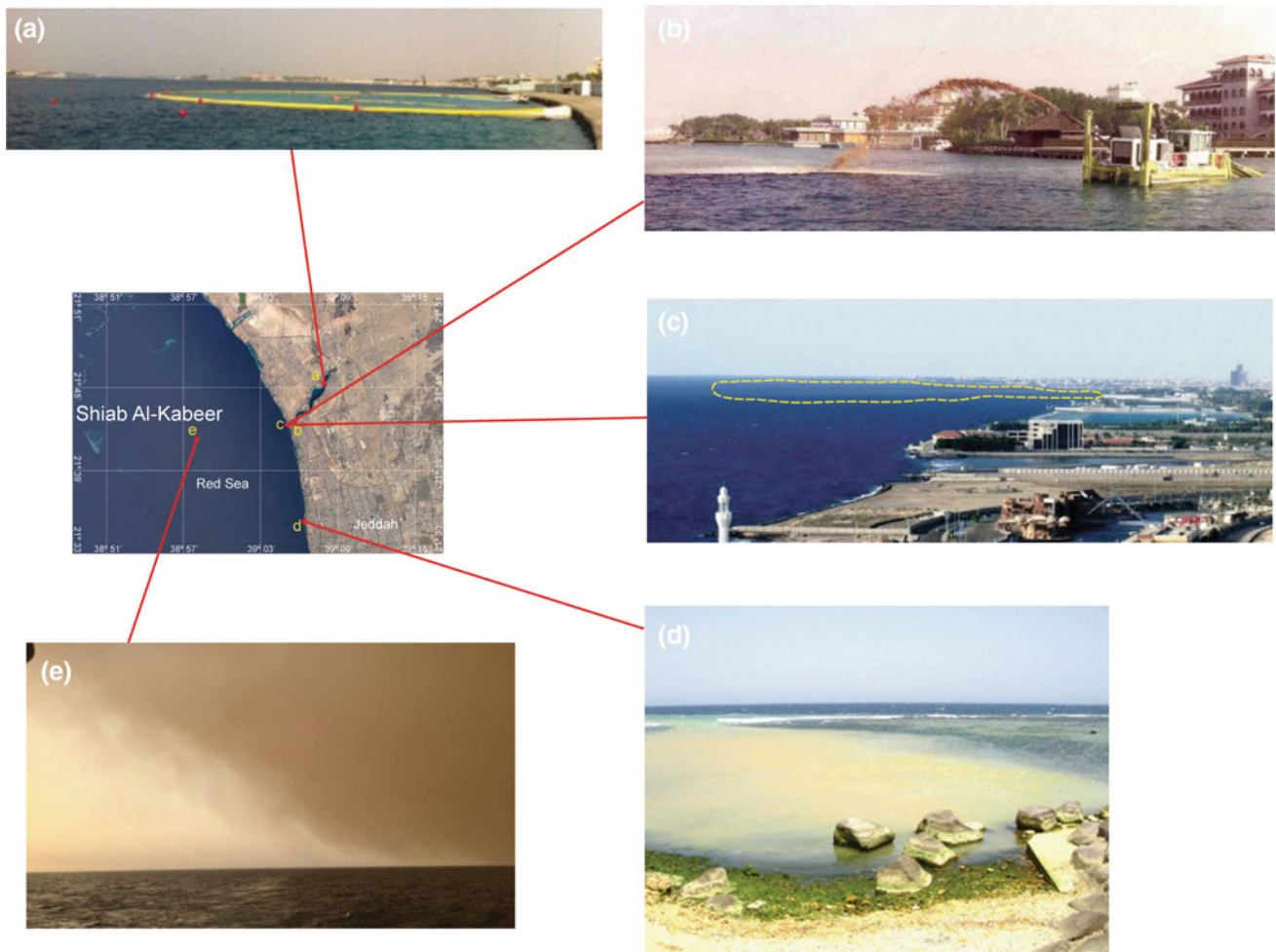
Fig. 19 Probable modes of sediment input to the shoal. a Floaters (in yellow) deployed to restrict the effect of sediment plumes on the sharm, although the plume is eventually dispersed to the open sea by the surface current; b Dredging to increase the water depth for deep-keel boats to manoeuvre easily. The dredged material is dumped into the deeper water regardless of the environmental hazard or impact; c sediment plume from Sharm Obhur moving in a westerly direction. This event is after rainfall; d inadequately treated sewage and ground
