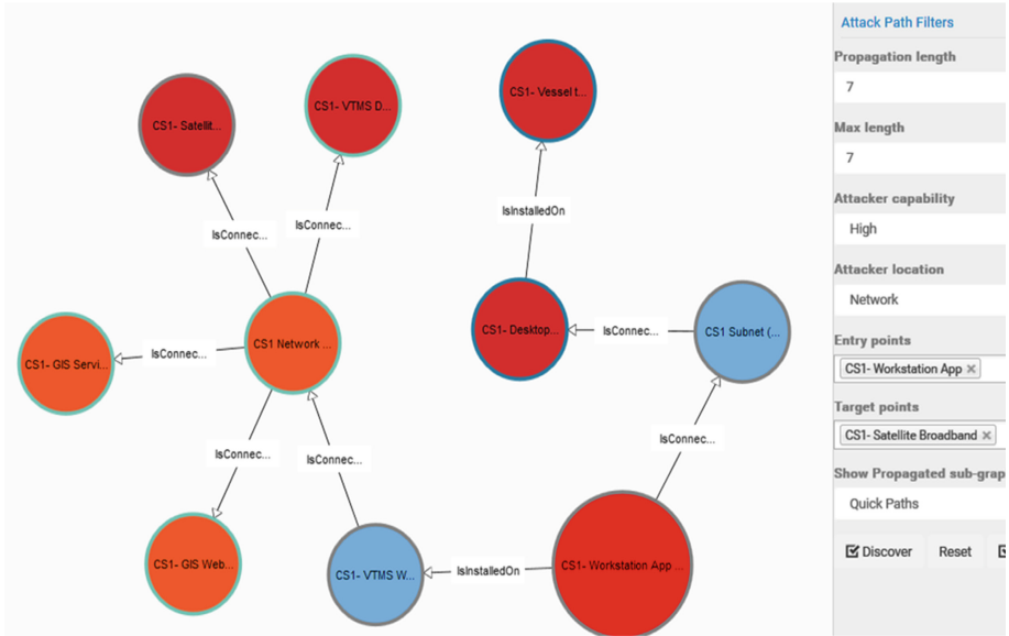
Fig. 2. An attack-path query depicting how skilled hacker terrorists can launch a series of cyber-attacks to the VTMS of the Cruise Service infrastructure; starting from a simple domain user workstation, ending up to satellite modem penetration and closure.
