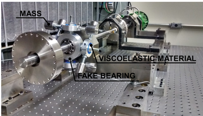
Fig. 7. Rotor assembled with compact angular VDN compound with C-1002.
