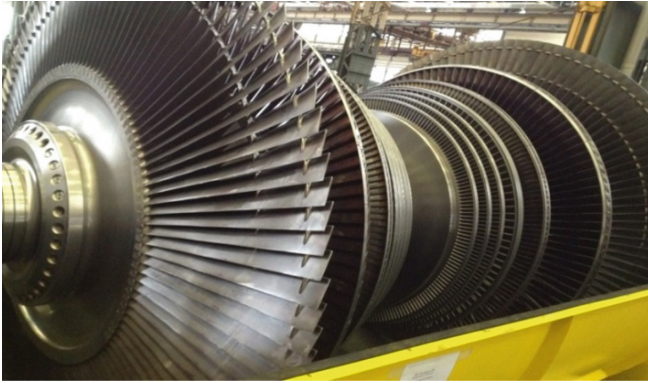
Fig. 3. Double flow low pressure steam turbine rotor after finishing at factory
