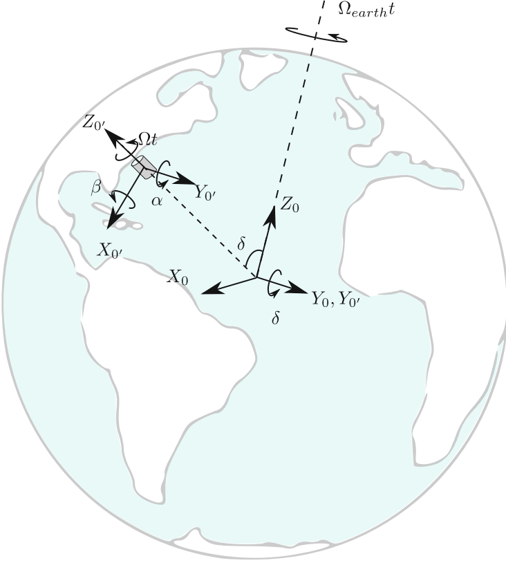
Fig. 1. Sketch of a FESS (illustrated as a cylinder) located at the surface of the earth.
