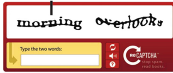
Fig. 1. Google’s RECAPTCHA [20] include a distorted word and a word scanned from a book, it also adds interference lines. Users need to enter two words together would they be able to approve.
