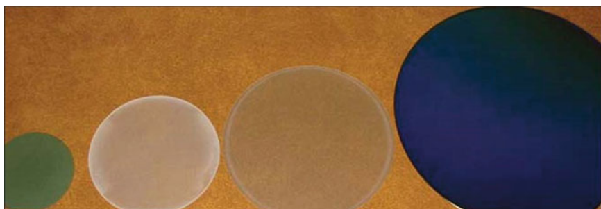
Fig. 1.16 HVPE-AlN templates by TDI Inc. (2 in. AlN-on-sapphire, 3 in. AlN-on-sapphire, 4 in. GaN-on-sapphire, and 6 in. AlN-on-Si from left to right)
