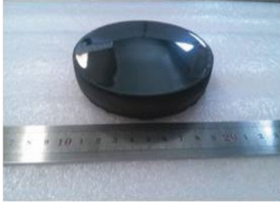
Fig. 2.9 Photograph of 4 in. 4H-SiC single crystal (Provided by Dr. Peng Y at Shandong University)
