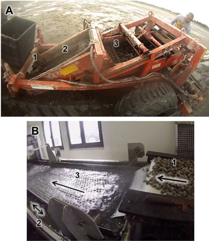
Fig. 14.9 (a) Manila clam ( Tapes philippinarum ) harvesting using a tractor-drawn rig which scoops the top few centimeters of mudflat (1), conveying the sediment and clams (2) to a flat, oscillating mesh (3), which allows the sediment and sub-sized clams to be returned to the mudflat. (b) Mechanized sorting of harvested clams. The clams are conveyed (1) to a submerged shaking mesh (2), which moves the clams forward (3). The holes in the mesh increase in size distally, so that the smaller clams fall through the mesh first; the larger clams fall through more distally, allowing them to be size-graded. Chellet-Bertheau Productions Ltd., Le Croisic, France. Photo Stewart Beattie.
