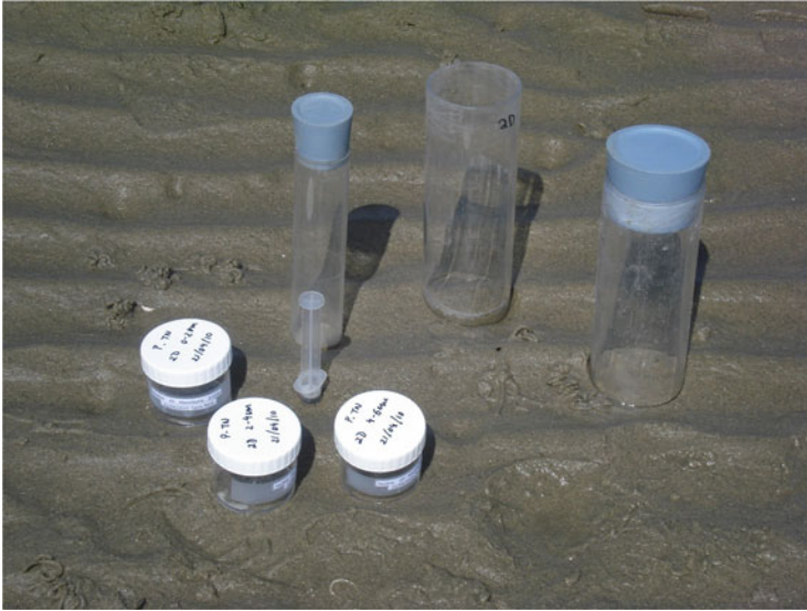
Fig. 5.2 Sampling equipment for meiofauna field sampling. Perspex hand corers with air-tight stoppers, a ‘microcore’ with a piston (here simply a sawn-off syringe) and recipients for sample storage. Photo by Tania Campinas Bezerra.
