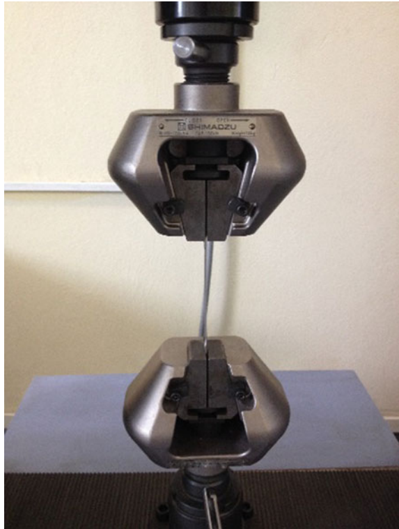
Fig. 13.4 Tension test for mechanical characterization
