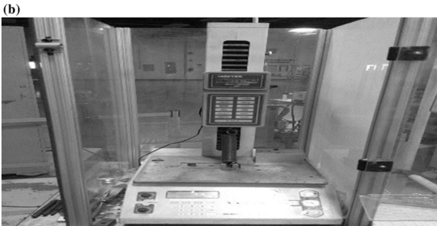
Fig. 14.5 a Partial drawing of the crimping machine, b Pulling testing equipment used for these experiments
