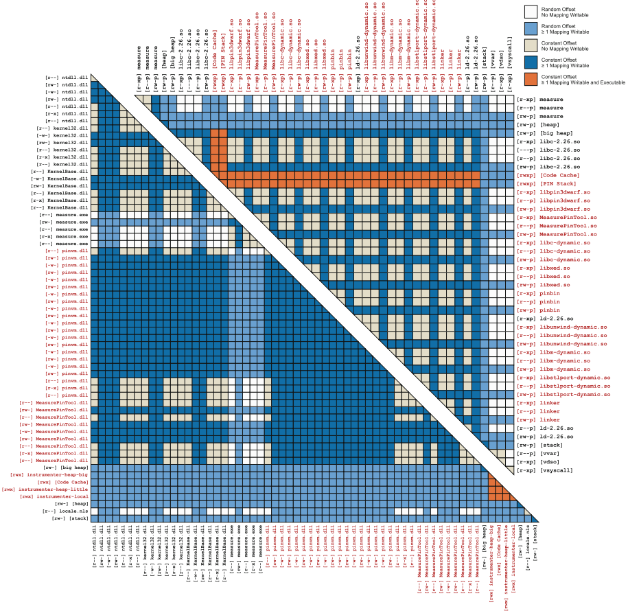
Fig. 3. Color matrices showing memory regions sharing random (□/■) or constant (□/■/■) distances with each other for applications instrumented by Linux (above right) and Windows (down left) version of Pin. The region names in red are additional components added by the instrumentation framework while in black are presented the program's original mapped files. (Color figure online)
