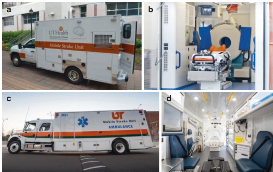
Fig. 35.1 Mobile stroke units in the United States: original vs. newer imaging technology. (a) University of Texas at Houston (UT-H), 1st MSU in the USA; (b) Interior of UT-H MSU with CereTom® computed tomography (CT) system; (c) University of Tennessee Health Sciences Center (UTHSC) MSU; (d) Interior of UT-M MSU with Siemens SOMATOM® Scope CT system
