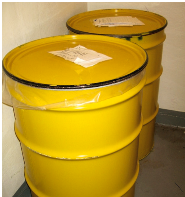
Fig. 7 A lead-shielded waste container used for the storage and disposal of photon emitters such as positron-emitting radionuclides
