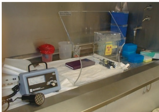
Fig. 5 An acrylic glass setup commonly used for the shielding of beta particles in a laboratory
